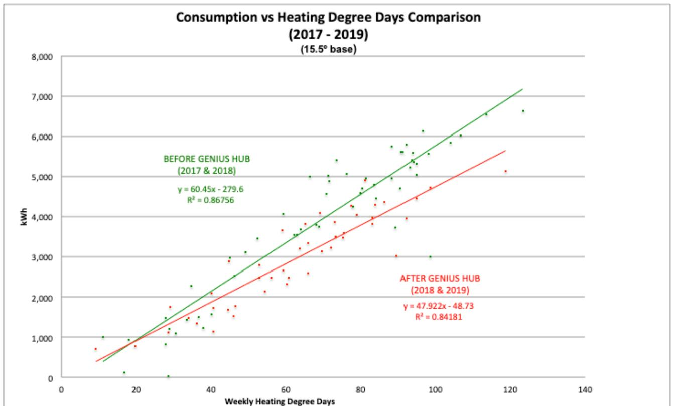
**Figure 8** - Graph comparing energy consumption per weekly heating degree days before and after installation of the Genius Hub (Figures 3 & 7 augmented).
