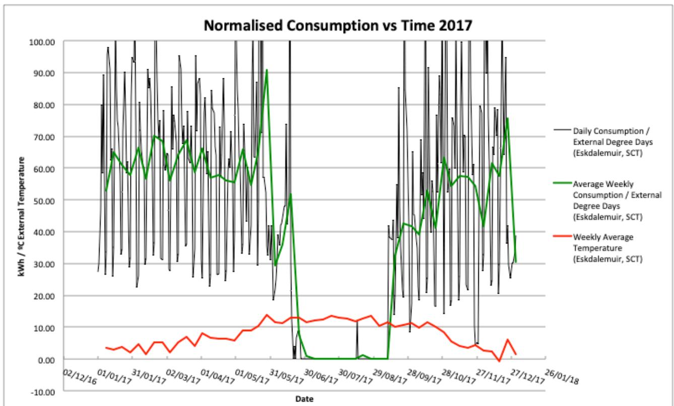
**Figure 2** – Graph showing Normalised Consumption vs Time (2017). The external temperature is shown in red.
