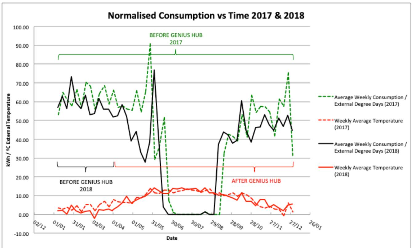
Figure 6 – Normalised consumption vs Time (2017 & 2018) (Figures 2 & 5 augmented).
