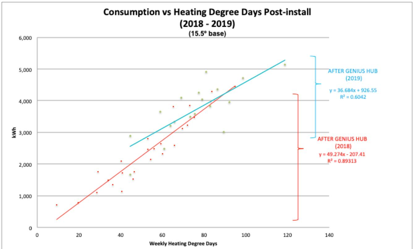
**Figure 7** – Graph showing energy consumption per weekly heating degree days after installation of the Genius Hub system (01/04/2018 -> 01/05/2019).
