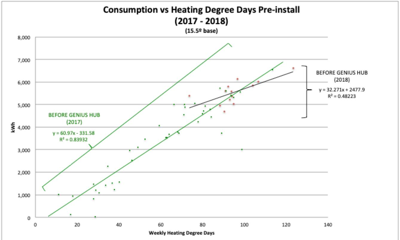
**Figure 3** – Graph showing energy consumption per weekly heating degree days prior to installation of Genius Hub system (01/01/2017 -> 31/03/2018).
