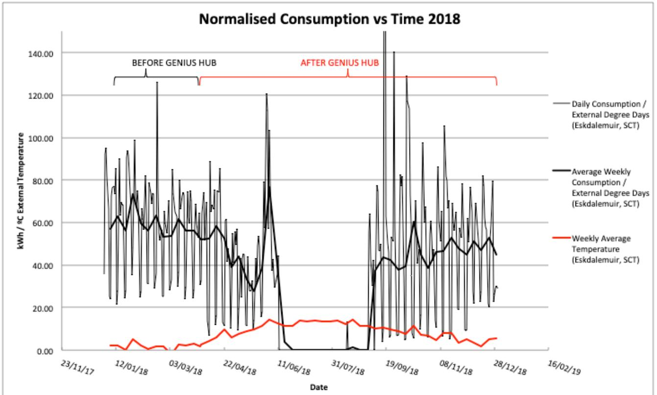
Figure 5 - Normalised Consumption vs Time (2018).
