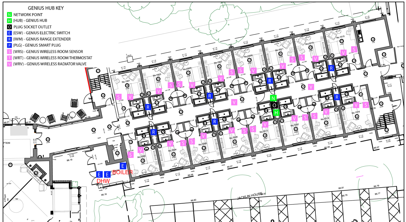
Figure 4 - Example of ground floor installation of Genius Hub
