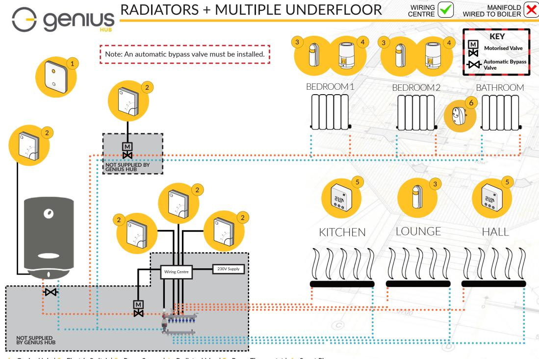
1 - Genius Hub | 2 - Electric Switch | 3 - Room Sensor | 4 - Radiator Valve | 5 - Room Thermostat | 6 - Smart Plug
