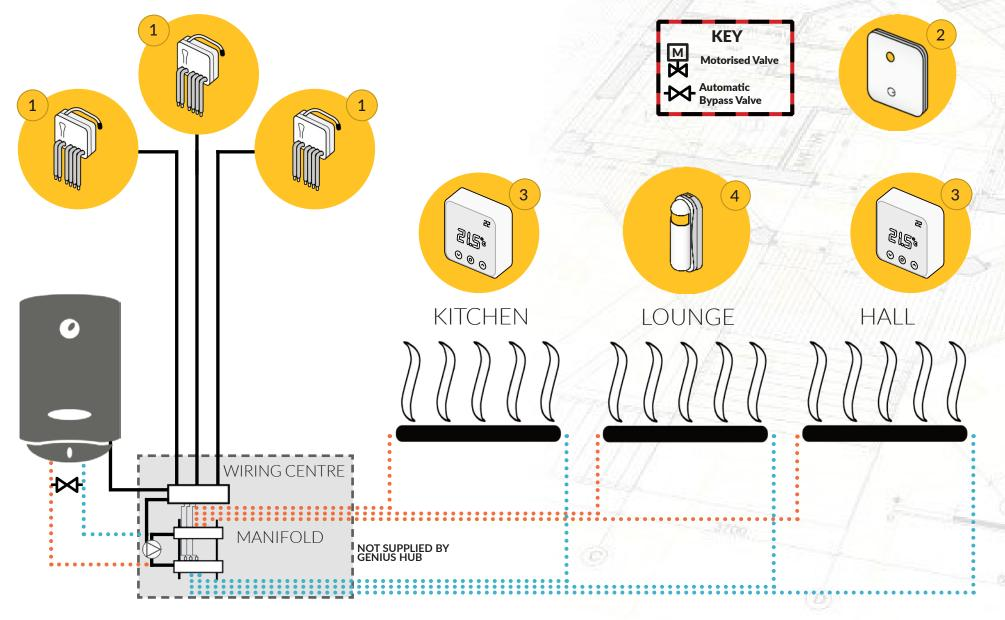
1 - Electric Relay | 2 - Genius Hub | 3 - Room Thermostat | 4 - Room Sensor
