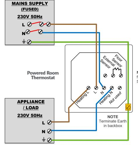
**NOTE** Insert link or floor probe into Floor Sensor terminals
