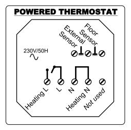
**NOTE** If the appliance/load has a fused spur then this needs to be retained. The Powered Thermostat should be wired in line with any existing fused spur.
