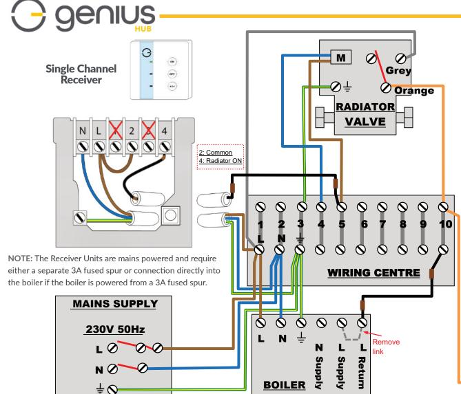
NOTE: The Underfloor Wiring Centre **UFH SUPPLY** terminals for the Zone Valve and Manifold Pump are Volt-Free. 230V 50Hz Grev Orange **UFH VALVE UFH PUMP** Maximum pump rating: 0.6A
