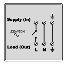
**NOTE** The Electric Switch is mains powered and requires either a separate 3A fused spur or connection directly into the boiler if the boiler is powered from a 3A fused spur.
