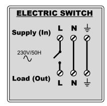
**NOTE:** If the appliance/load has a fused spur then this needs to be retained. The Electric Switch should be wired in line with any existing fused spur.
