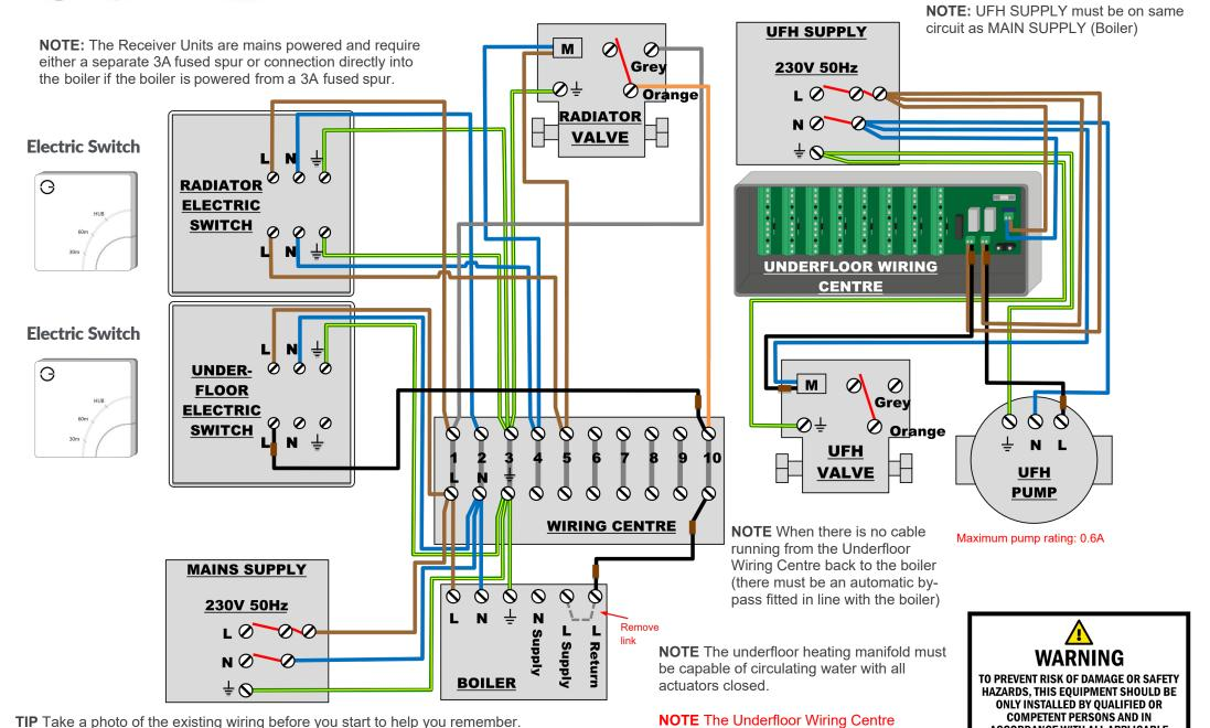
terminals for the Zone Valve and Manifold
